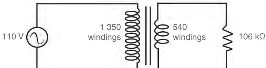
1.1 Calculate the tension in the secondary coil.
